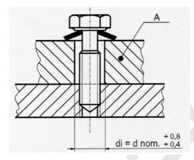
Torque tightening is carried out so that a pre-load, between 80 and 90 % of the elastic limit of the screw to which the washer is incorporated, is induced after calibration on a rig for the measurement of the torque/pre-loads.
